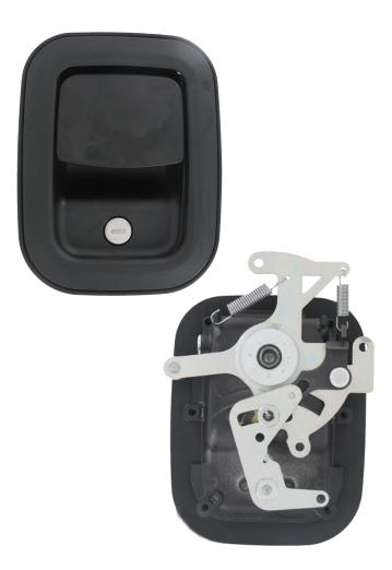
This flush mounted paddle handle with free-floating paddle (when locked) is a redesign of our popular 030-0875 Flush Mounted Paddle Handle. Containing an update to the mechanical design and with a modernized look, it can be used in FMVSS 206 applications, is power lockable and features same four point pivot plate and lock cam actuation.
